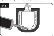
Apply sikaflex around cable holder and on the top of the screws for waterproof
