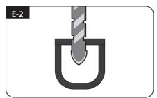
Drill a 25mm hole (or larger) in the centre of the tape marking
