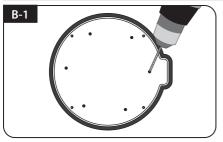
Place the mounting plate on the sikaflex and make 6 holes (2mm) with a power drill
