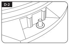
Place the antenna and deflector on the aluminium plate and put the washers over each bolt
