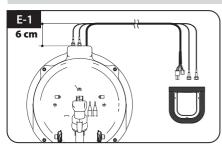
Connect signal cable to antenna, place cable holder and apply electrical tape 5mm from the outside of the cable holder
