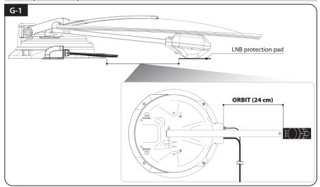
Attach LNB protection pad, placing one end by 24cm away from antenna port. Check that LNB bracket sits on the pad properly and does not touch cables when home positioning
