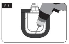
Place the assembled cable holder inside the tape markings. Drill three(3) 2mm holes
