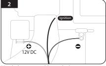
Match the power cables to the battery polarities, red-red, black-black and yellow ignition cable- ignition port of the vehicle
